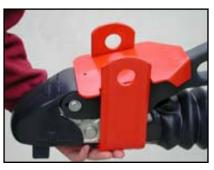
3. Place steel shield plate over the handle.
