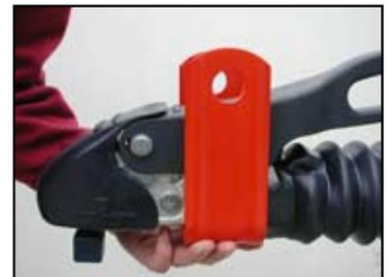
2. Pass up Hitchlock from beneath the coupling head ensuring front fixing bolt fits inside. **Note:** A cut out is provided where a rear vertical bolt fixing is used.
