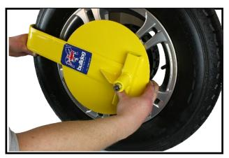
With the lock in the unlocked position, fit the top arm and rotate until it is vertical.
