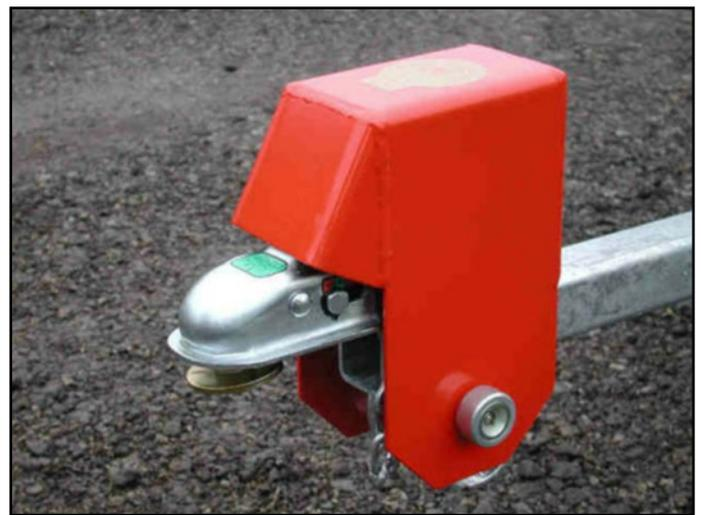
Lower the cover over the hitch handle. Insert lock bolt through both holes of the cover. Fit the recessed cup over end of lock bolt, then turn key a quarter turn to lock and remove key.
