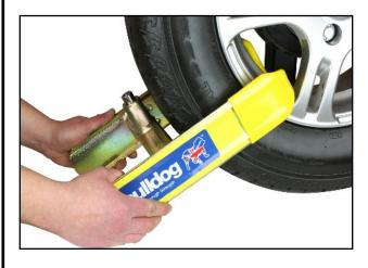
**3.** Slide inner and outer arms together, ensuring pointed outer arm fits into recess or hole in wheel, and push lock into nearest hole.
